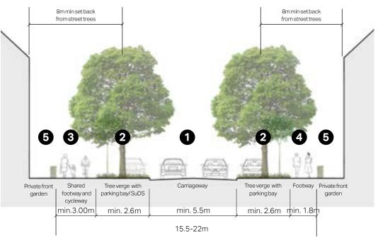
Figure 29: Section showing indicative dimensions for primary roads.
