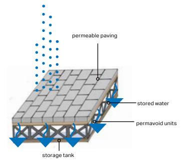
Figure 61: Diagram illustrating the functioning of a soak away
