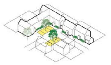
Figure 38: Illustrative diagram showing an indicative layout of parking courtyards.
