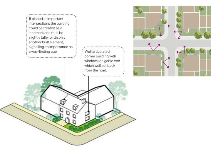
Figure 48: Diagram reflecting design principles for corner buildings.
