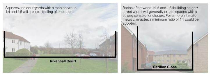
Figure 49: The various enclosure ratios depend on the amount of front garden width, road width, tree canopies and building heights.
