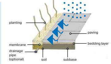
Figure 66: Diagram illustrating the functioning of a soak away garden
