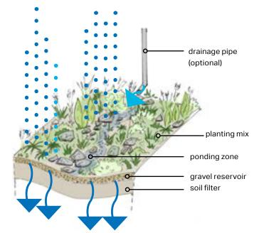
Figure 65: Diagram illustrating the functioning of a rain garden
