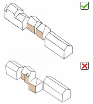
Figure 45: New buildings should respect the established building line.
