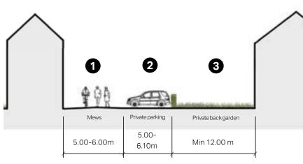
Figure 31: Section showing indicative dimensions for mews. The mews width may vary to discourage speeding or provide space for parking.
